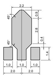
RemarkThe mounting pad layout in this document is for reference only.When designing PCB, please consider workability of mounting, solder joint reliability, prevention of solder<br/>bridge and so on, in order to optimize the design.
