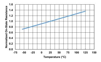
Figure 14. Normalized On-State Resistance
