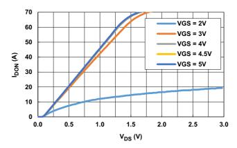
Figure 4. Output Characteristics (+125°C)
