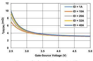
Figure 7. On-State Resistance (+25°C)
