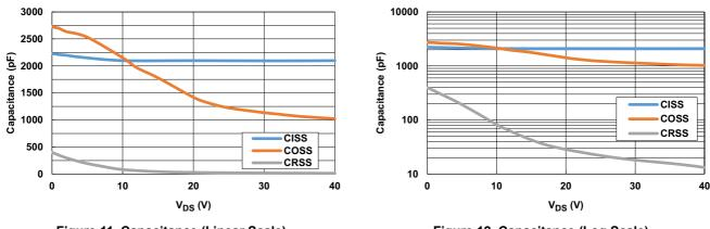
Figure 11. Capacitance (Linear Scale)
