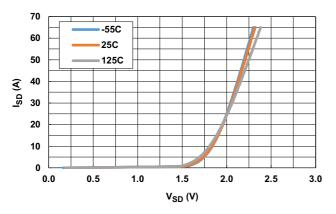
Figure 13. Reverse Drain-Source Characteristics
