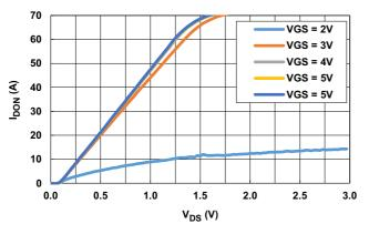
Figure 3. Output Characteristics (+25°C)
