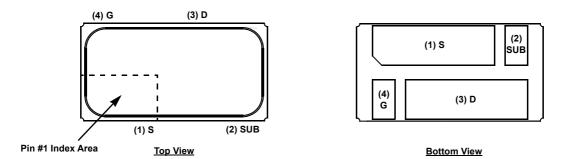
Note: The ESD triangular mark indicates Pin #1. It is a part of the device marking and is placed on the lid in the quadrant where Pin #1 is located.
