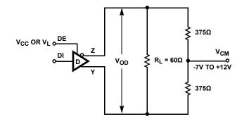
FIGURE 1B. VOD WITH COMMON MODE LOAD
