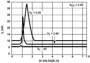
FIGURE 9. VL SUPPLY CURRENT vs LOGIC PIN VOLTAGE
