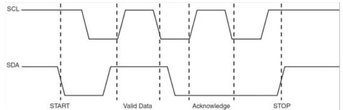
**Figure 1: Standard I<sup>2</sup>C Transaction**
