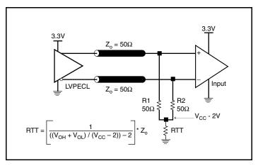
Figure 4A. 3.3V LVPECL Output Termination
