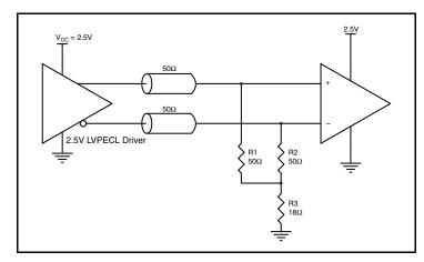
Figure 5B. 2.5V LVPECL Driver Termination Example
