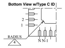
There are 2 methods of indicating pin 1 corner at the back of the VFQFN package are:
