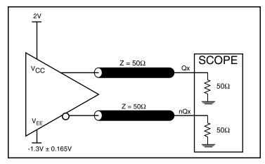
3.3V LVPECL Output Load AC Test Circuit
