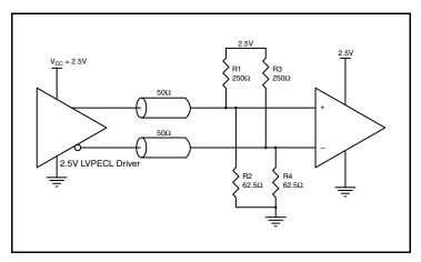
Figure 5A. 2.5V LVPECL Driver Termination Example
