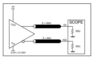
2.5V LVPECL Output Load AC Test Circuit
