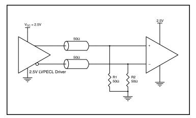
Figure 5C. 2.5V LVPECL Driver Termination Example
