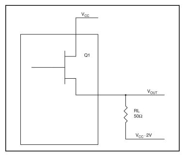
Figure 6. LVPECL Driver Circuit and Termination
