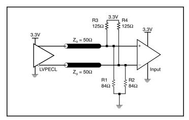
Figure 4B. 3.3V LVPECL Output Termination
