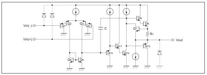
Note: If Input/Output terminals voltage over the absolute maximum ratings, there is possibility of mis-operation, characteristics deterioration and destruction, because of the current's flowing to parasitic diode in IC. The Input/Output terminals are recommended to be protected with the clamp circuit which using the diode with low forward voltage (like schottky barrier diode) when there is a possibility for the Input/Output terminals voltage exceeds the absolute maximum ratings.
