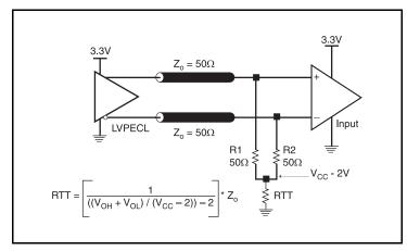
Figure 1A. 3.3V LVPECL Output Termination
