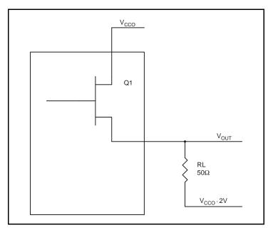
Figure 4. LVPECL Driver Circuit and Termination
