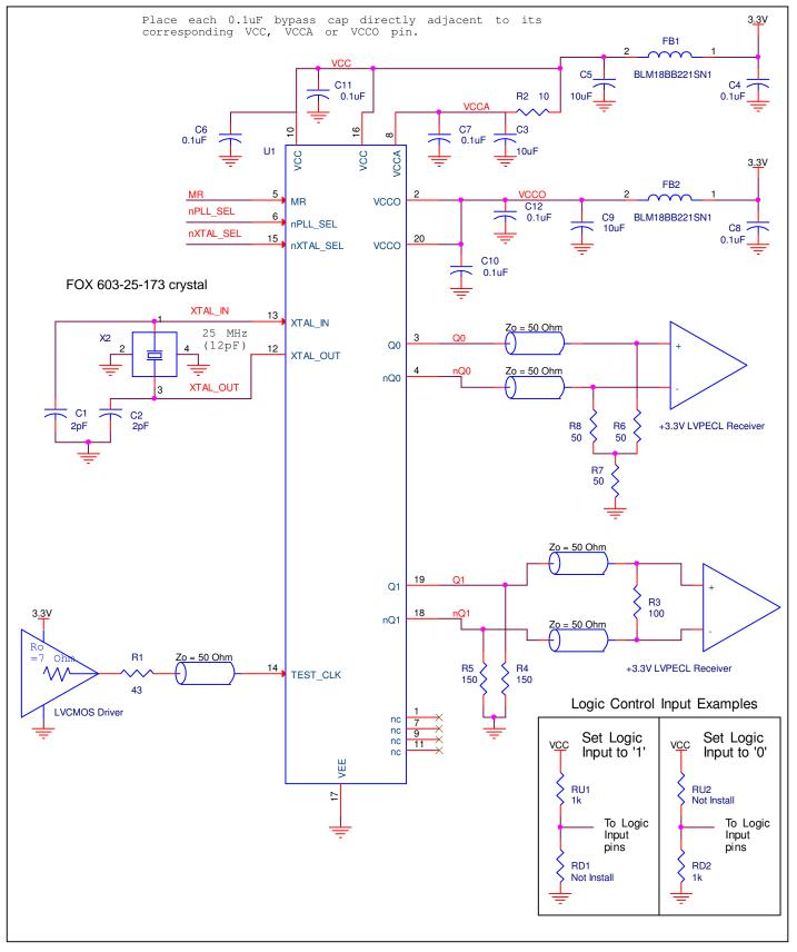
Figure 3. 8V43042 Schematic Example
