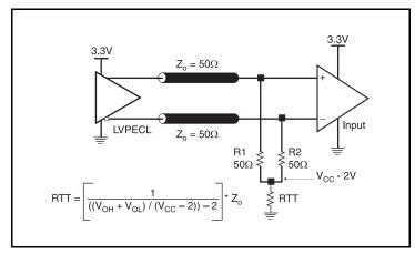
Figure 1A. 3.3V LVPECL Output Termination
