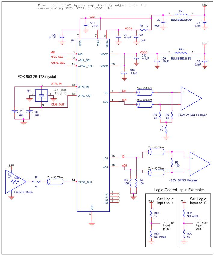
Figure 3. 8V43042 Schematic Example
