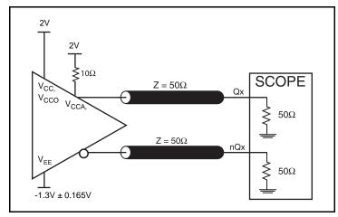
3.3V LVPECL Output Load Test Circuit
