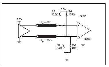
Figure 1B. 3.3V LVPECL Output Termination
