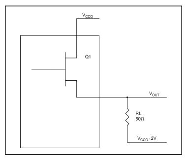
Figure 4. LVPECL Driver Circuit and Termination
