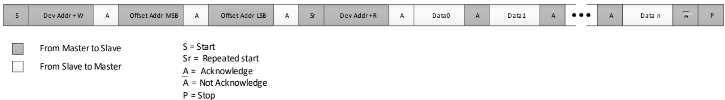
Figure 22. Master I 2 C Initialization Mode
