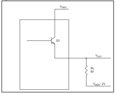
To calculate power dissipation per output pair due to loading, use the following equations which assume a 50 $\Omega$  load, and a termination voltage of V<sub>DDO</sub> – 2V.
