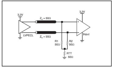
Figure 16: 3.3V LVPECL Output Termination
