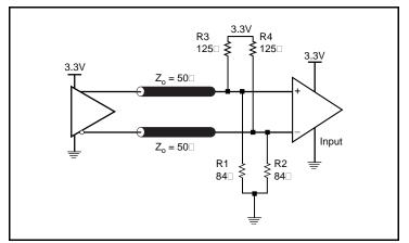
Figure 17: 3.3V LVPECL Output Termination
