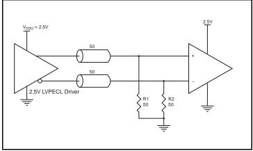
Figure 19: 2.5V LVPECL Driver Termination Example
