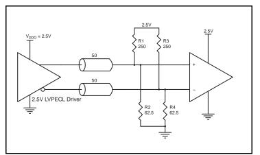
Figure 18: 2.5V LVPECL Driver Termination Example
