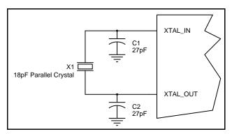
Figure 1: Crystal Input Interface
