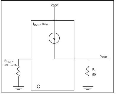
HCSL is a current steering output which sources a maximum of 17mA of current per output. To calculate worst case on-chip power dissipation, use the following equations which assume a  $50\Omega$  load to ground.
