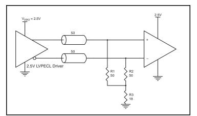
Figure 20: 2.5V LVPECL Driver Termination Example
