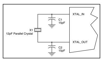
Figure 2: Crystal Input Interface
