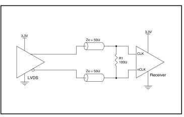
Figure 9: CLK/nCLK Input Driven by a 3.3V LVDS Driver
