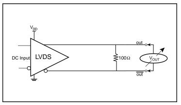
**Differential Output Voltage Setup**
