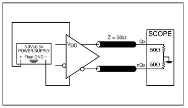
Output Load AC Test Circuit
