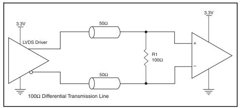
Figure 1. Typical LVDS Driver Termination
