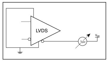
Power Off Leakage Setup
