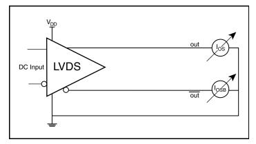
**Output Short Circuit Current Setup**
