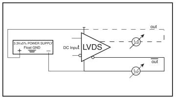
High Impedance Leakage Current Setup
