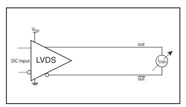
**Differential Output Short Circuit Setup**
