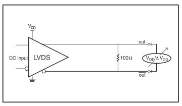
**Differential Output Voltage Setup**
