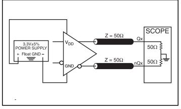
3.3V LVDS Output Load AC Test Circuit
