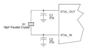
FIGURE 2. CRYSTAL INPUT INTERFACE
