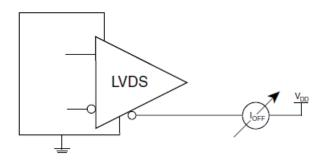
**OUTPUT SHORT CIRCUIT CURRENT SETUP**
