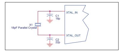
FIGURE 2. CRYSTAL INPUT INTERFACE
