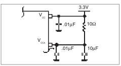
FIGURE 1. POWER SUPPLY FILTERING
