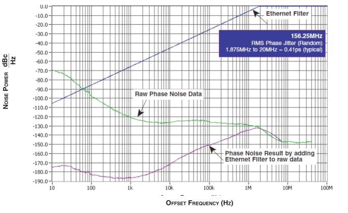
TYPICAL PHASE NOISE AT 156.25MHz @ 3.3V
