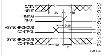
Set-up, Hold, and Release Times
