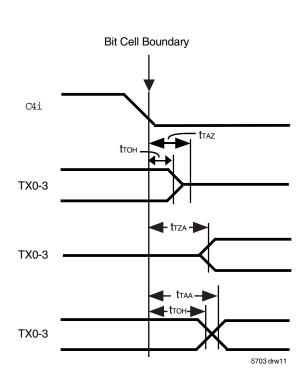
Figure 7. Serial Outputs and External Control
