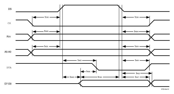
Figure 10. Processor Bus
