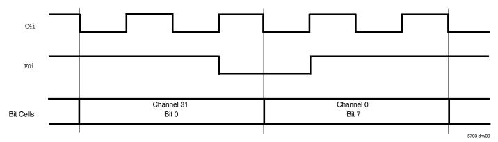
Figure 5. Frame Alignment
