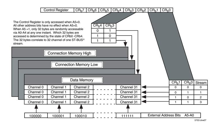
Figure 3. Address Mapping
