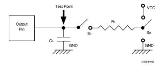
Figure 4. Output Load
