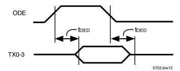
Figure 8. Output Driver Enable
