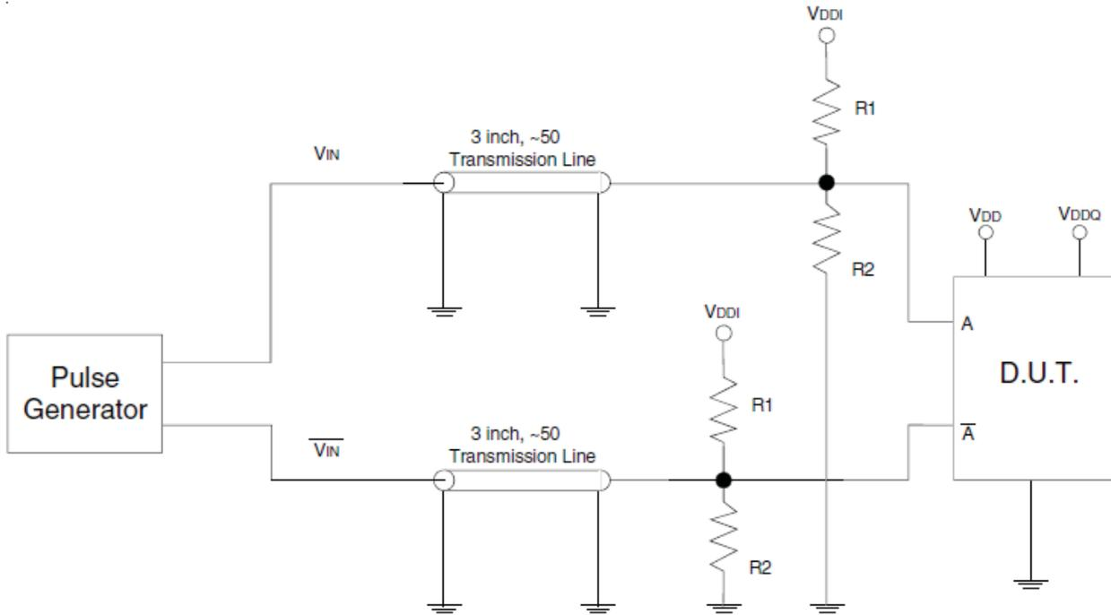
Test Circuit for Differential Input<sup>(1)</sup>
