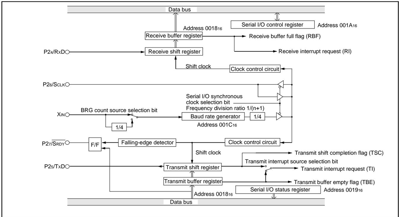
Fig. 14 Block diagram of clock synchronous serial I/O
