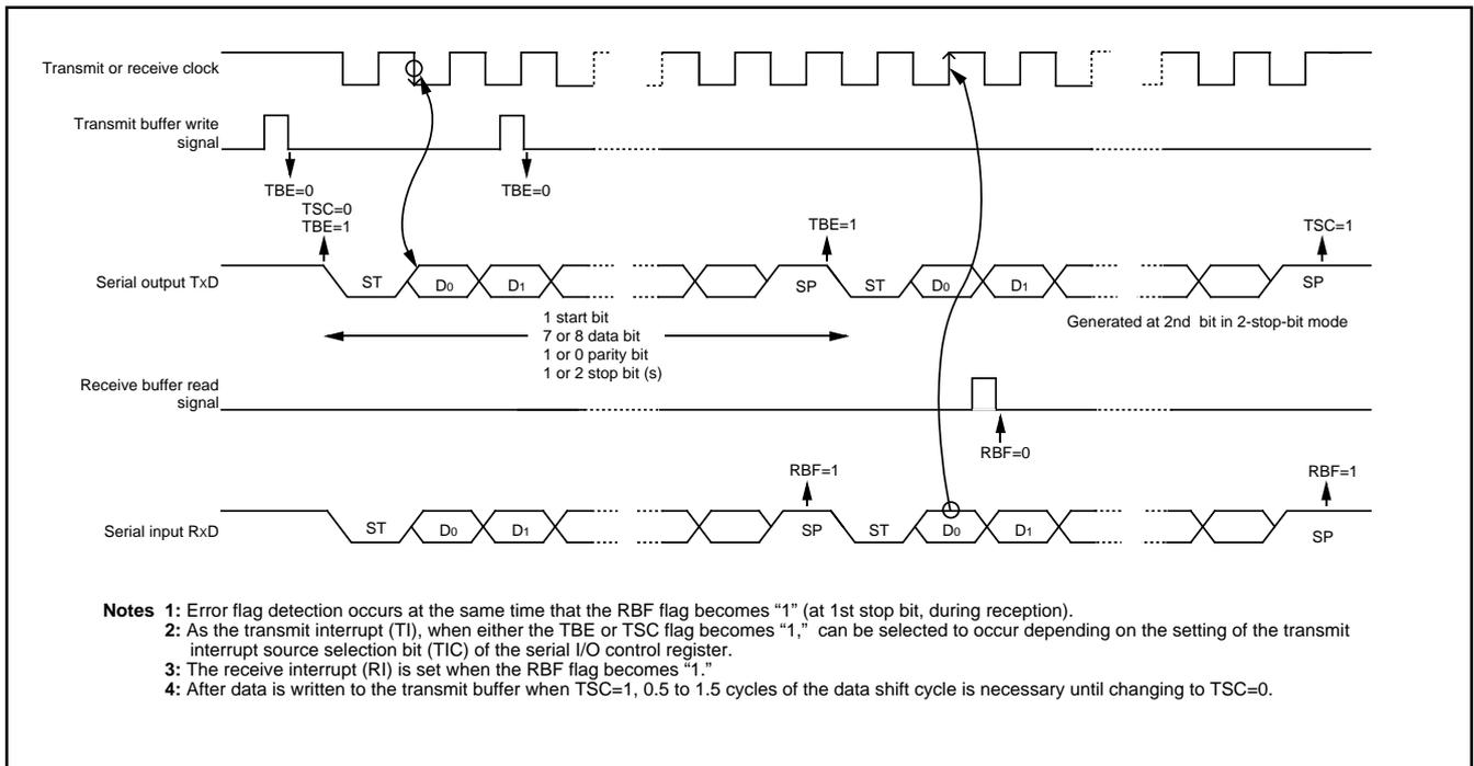
Fig. 17 Operation of UART serial I/O function
