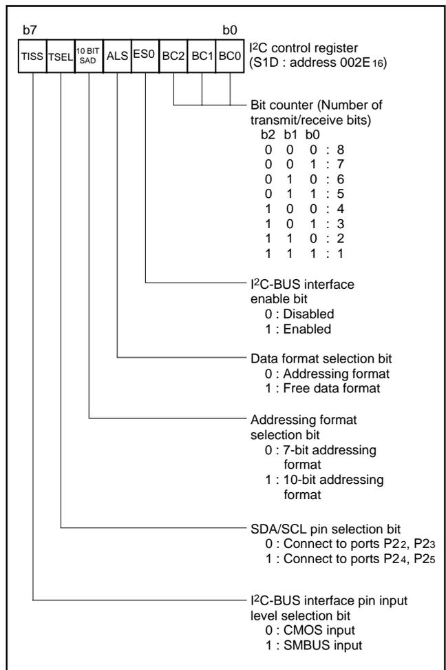
Fig. 23 Structure of I<sup>2</sup>C control register
