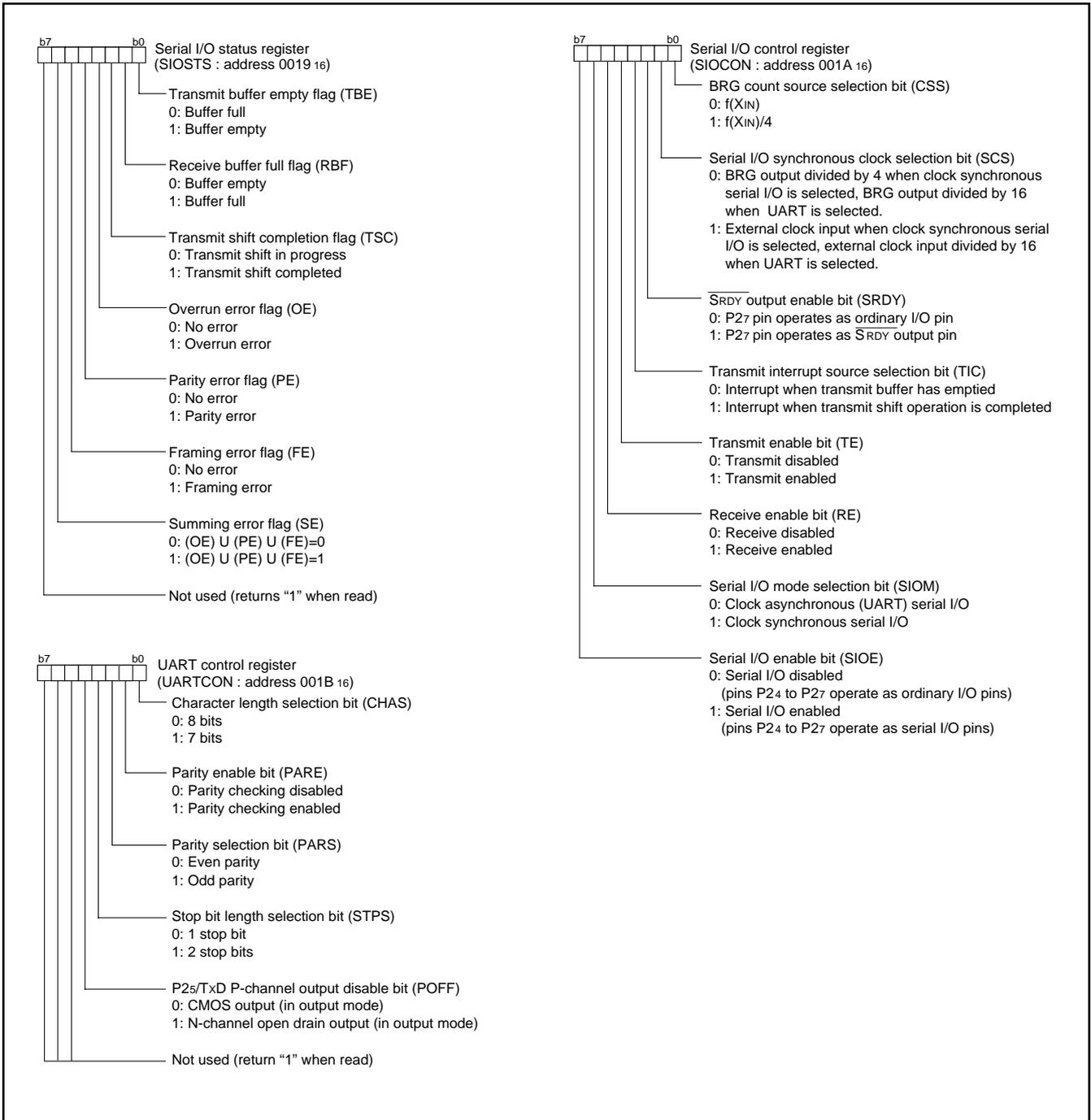
Fig. 18 Structure of serial I/O control registers
