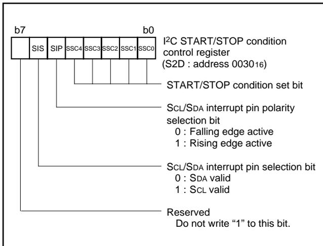
Fig. 30 Structure of I<sup>2</sup>C START/STOP condition control register
