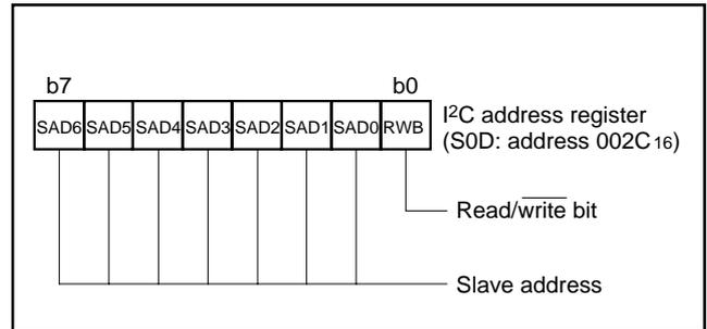
**Fig. 20 Structure of I<sup>2</sup>C address register**
