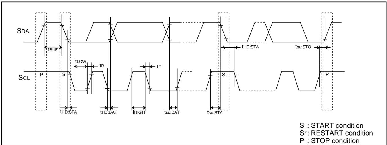
**Fig. 53 Timing diagram of multi-master I<sup>2</sup>C-BUS**
