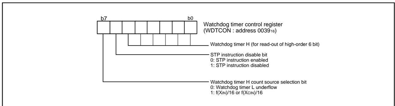
Fig. 40 Structure of Watchdog timer control register
