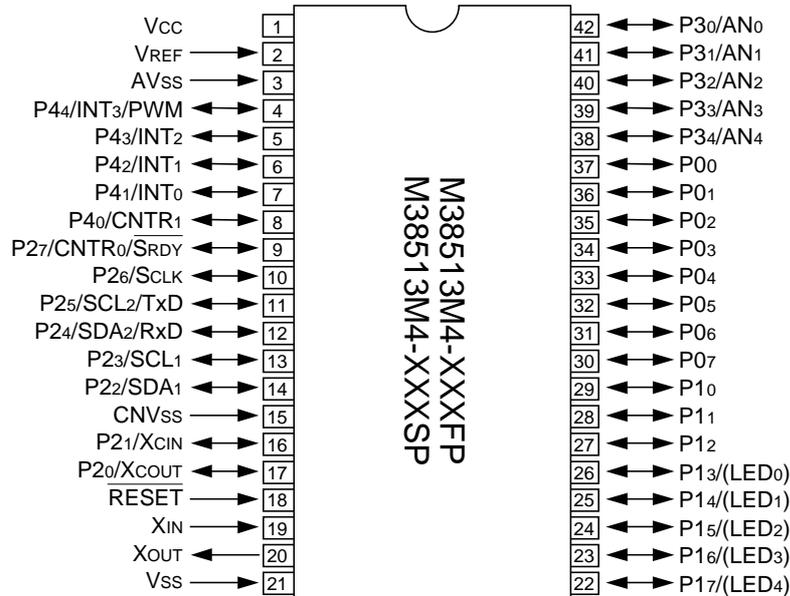
Package type : FP ..... 42P2R-A/E (42-pin plastic-molded SSOP)
