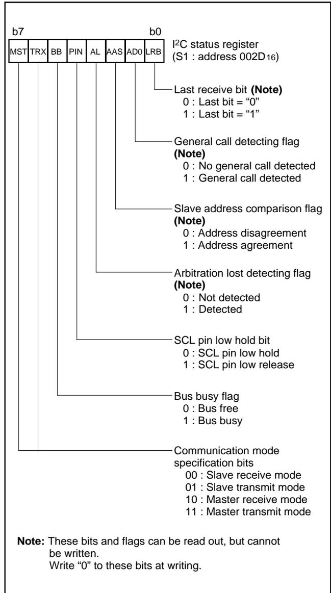
Fig. 24 Structure of I<sup>2</sup>C status register
