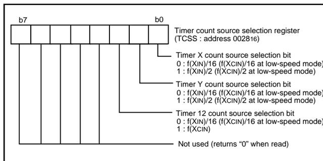
Fig. 12 Structure of timer count source selection register
