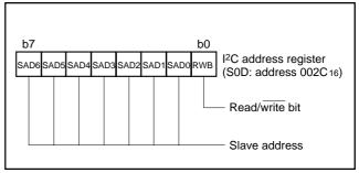
Fig. 20 Structure of I<sup>2</sup>C address register
