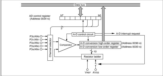
Fig. 38 Block diagram of A-D converter
