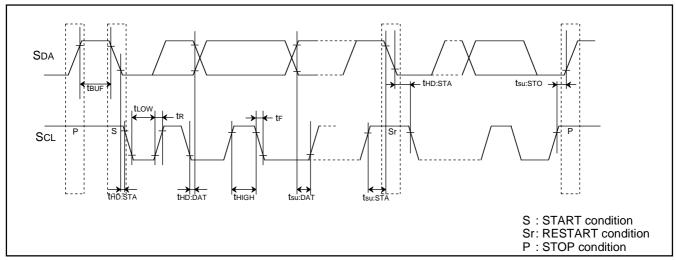
Fig. 53 Timing diagram of multi-master I<sup>2</sup>C-BUS
