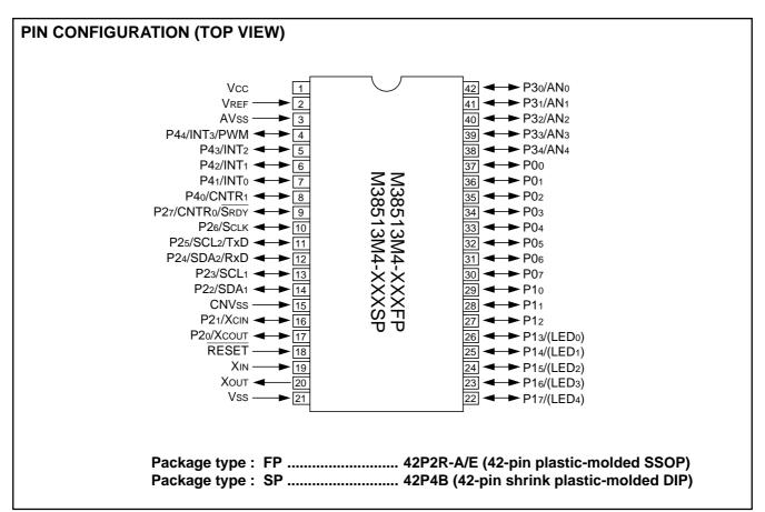
Fig. 1 M38513M4-XXXFP/SP pin configuration
