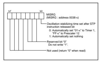
Fig. 46 Structure of MISRG
