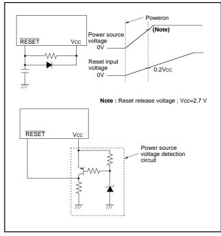
Fig. 41 Reset circuit example
