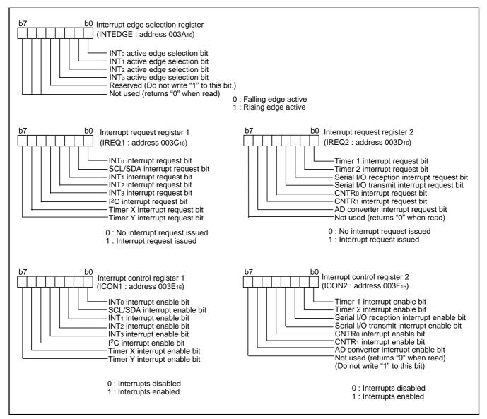
Fig. 10 Structure of interrupt-related registers (1)
