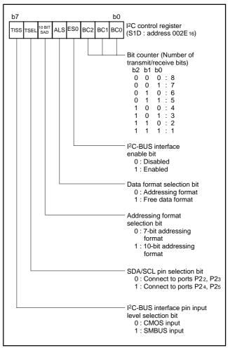
Fig. 23 Structure of I<sup>2</sup>C control register
