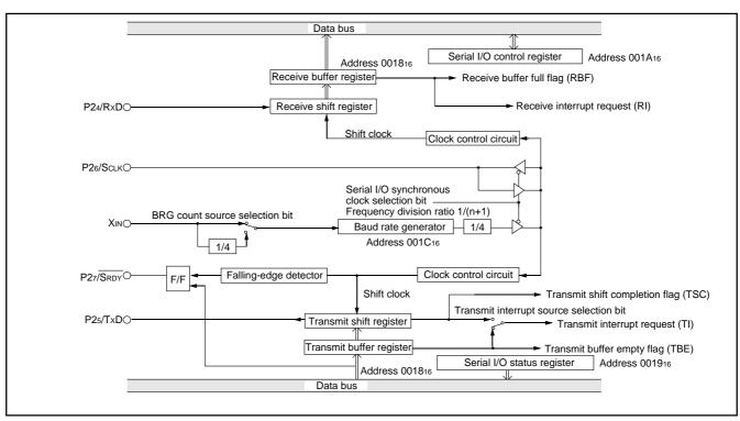
Fig. 14 Block diagram of clock synchronous serial I/O
