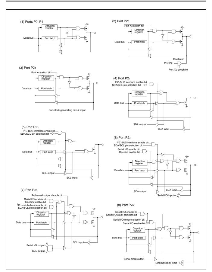
Fig. 7 Port block diagram (1)
