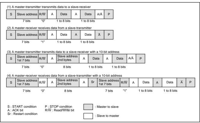
Fig. 31 Address data communication format
