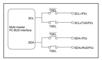
Fig. 22 SDA/SCL pin selection bit
