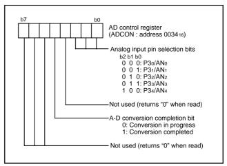
Fig. 36 Structure of AD control register
