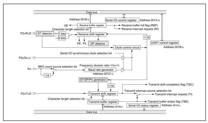
Fig.16 Block diagram of UART serial I/O
