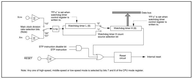
Fig. 39 Block diagram of Watchdog timer
