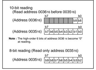
Fig. 37 Structure of A-D conversion registers
