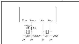
Fig. 44 Ceramic resonator circuit
