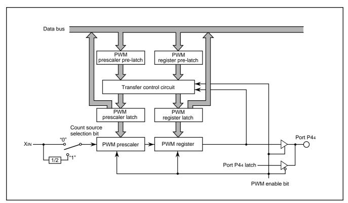
Fig. 33 Block diagram of PWM function
