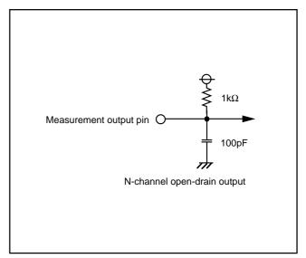
Fig. 51 Circuit for measuring output switching characteristics (2)
