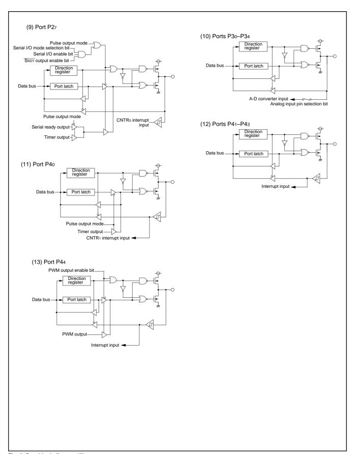
Fig. 8 Port block diagram (2)
