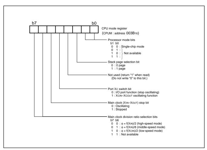
Fig. 4 Structure of CPU mode register
