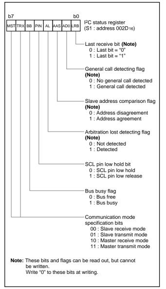
Fig. 24 Structure of I<sup>2</sup>C status register
