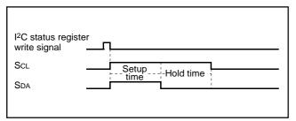
Fig. 26 START condition generating timing diagram
