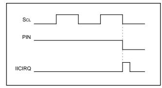
Fig. 25 Interrupt request signal generating timing
