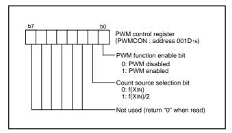
Fig. 34 Structure of PWM control register
