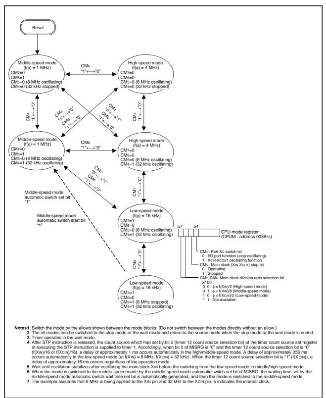
Fig 46. State transitions of system clock
