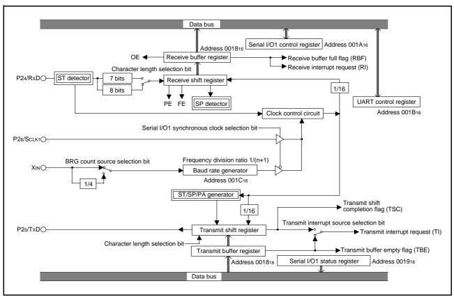
Fig 22. Block diagram of UART serial I/O1
