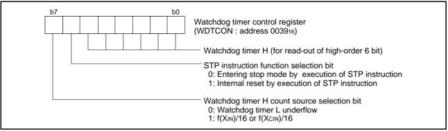
Fig 38. Structure of Watchdog timer control register
