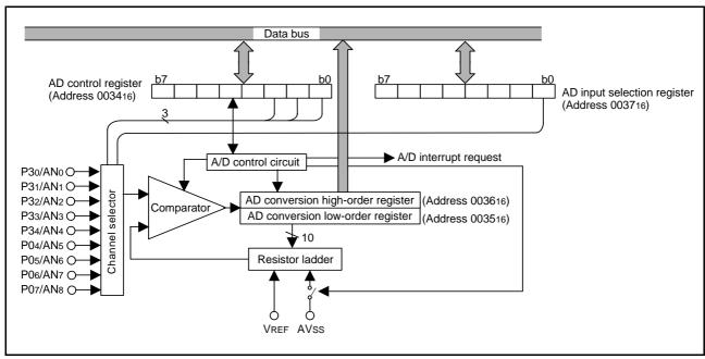
Fig 36. Block diagram of A/D converter
