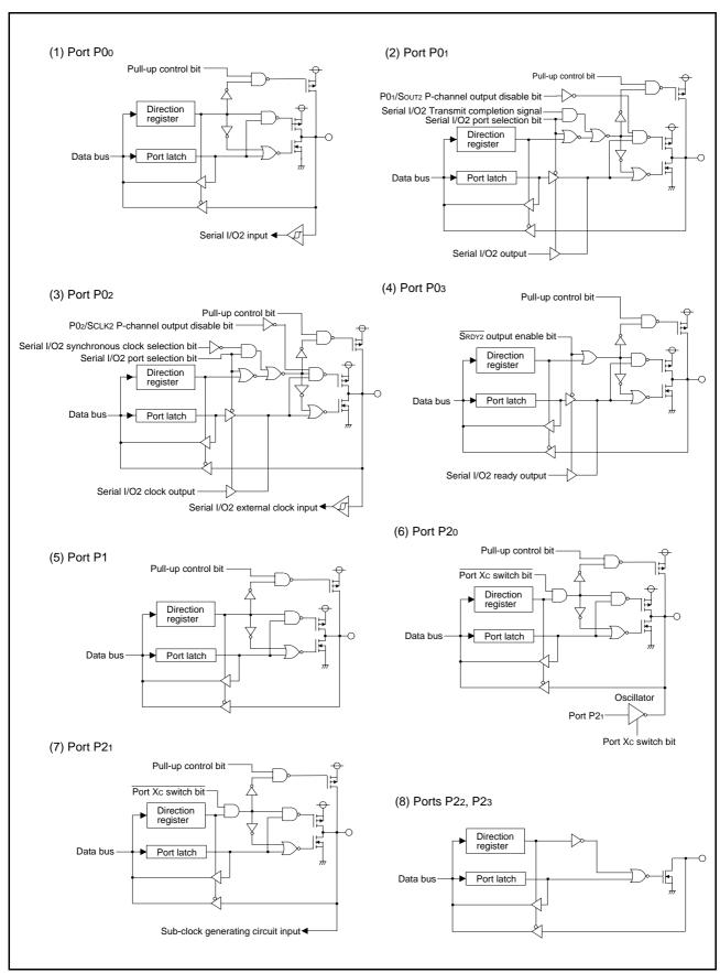
Fig 10. Port block diagram (1)
