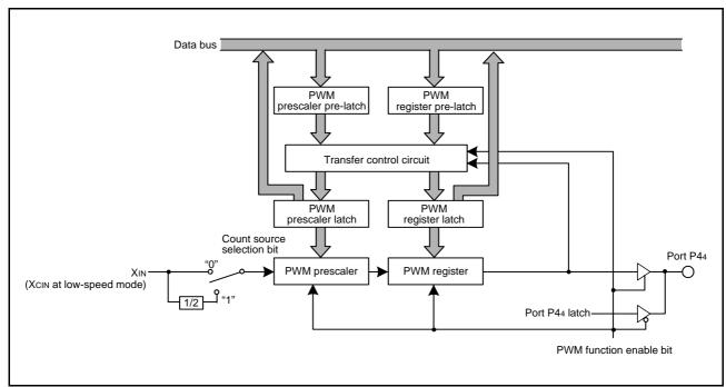
Fig 30. Block diagram of PWM function
