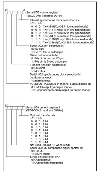
Fig 25. Structure of Serial I/O2 control registers 1, 2
