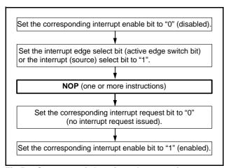
Fig 52. Sequence of changing relevant register
