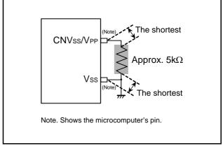
Fig 55. Wiring for the CNVss/VPP
