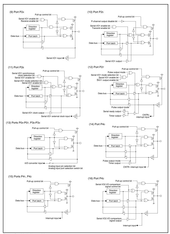
Fig 11. Port block diagram (2)
