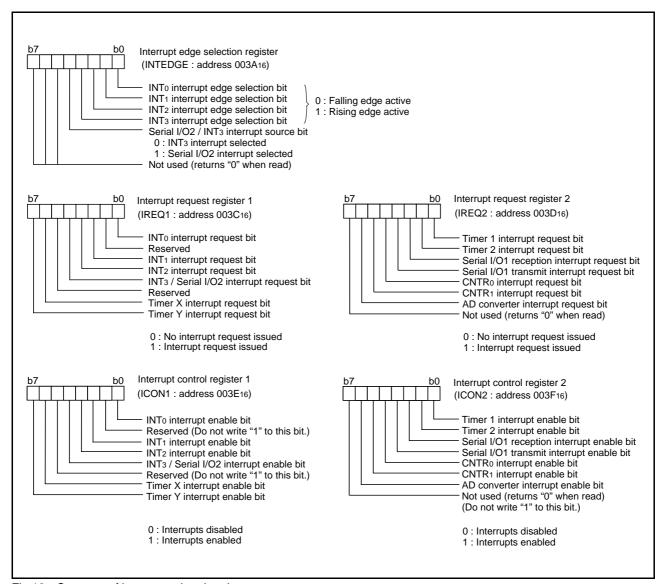
Fig 16. Structure of interrupt-related registers
