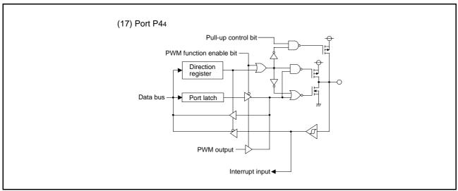
Fig 12. Port block diagram (3)
