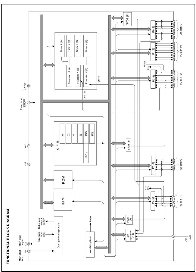
Fig 2. Functional block diagram
