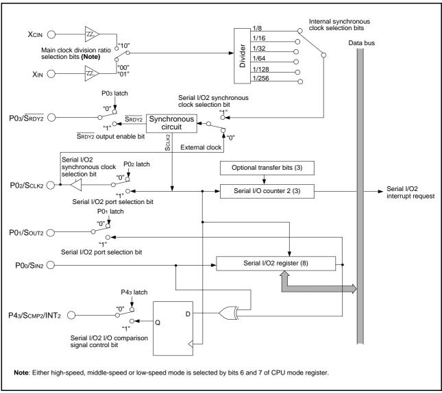
Fig 26. Block diagram of Serial I/O2
