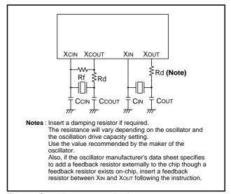
Fig 42. Ceramic resonator circuit
