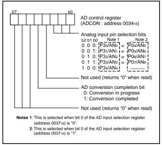
Fig 33. Structure of AD control register
