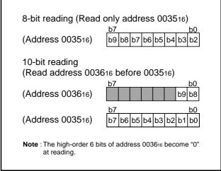
Fig 35. Structure of AD conversion registers
