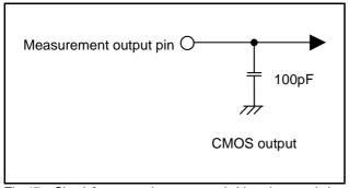
Fig 47. Circuit for measuring output switching characteristics
