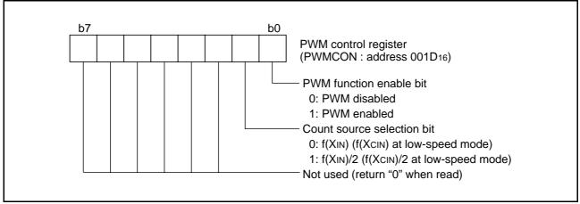
Fig 31. Structure of PWM control register
