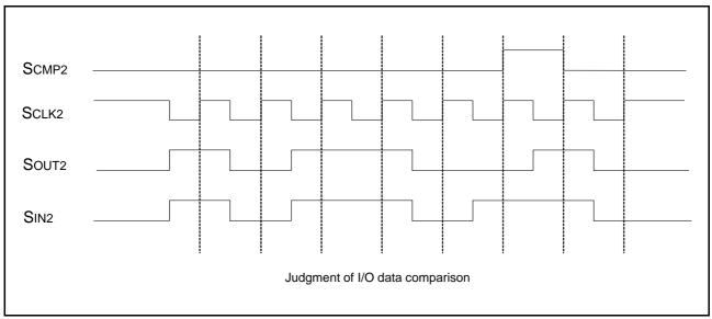
Fig 28. SCMP2 output operation
