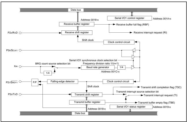
Fig 20. Block diagram of clock synchronous serial I/O1
