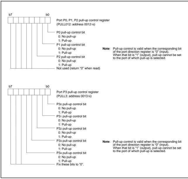
Fig 13. Structure of port registers (1)
