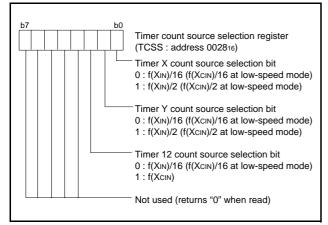
Fig 18. Structure of timer count source selection register
