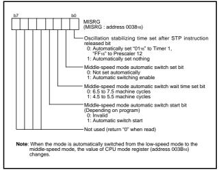
Fig 44. Structure of MISRG
