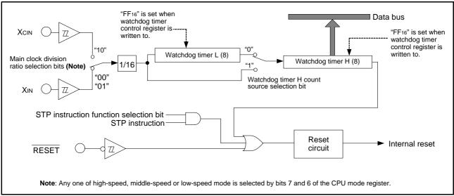
Fig 37. Block diagram of Watchdog timer
