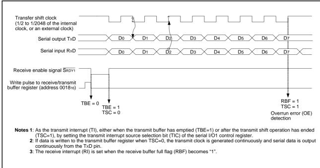
Fig 21. Operation of clock synchronous serial I/O1 function
