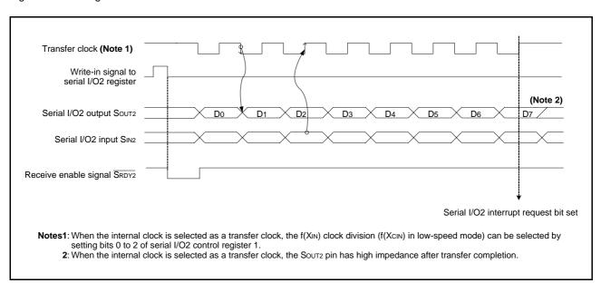
Fig 27. Timing chart of Serial I/O2
