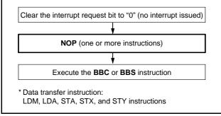
Fig 53. Sequence of check of interrupt request bit
