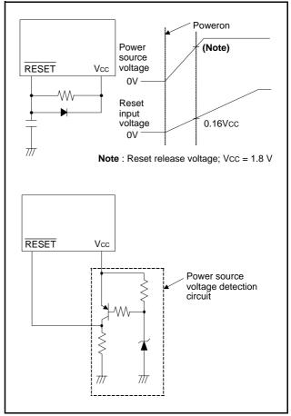
Fig 39. Reset circuit example
