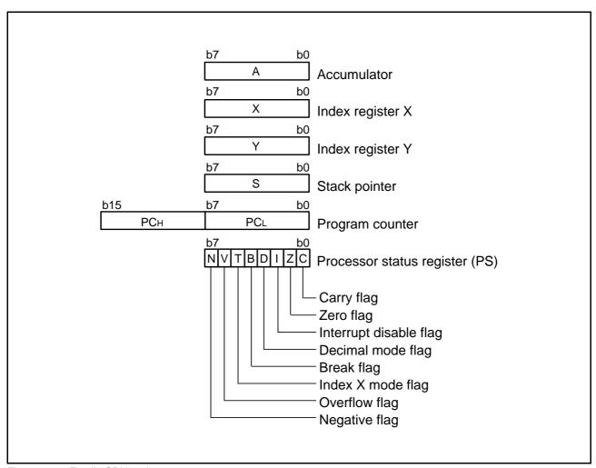
Fig 5. 740 Family CPU register structure
