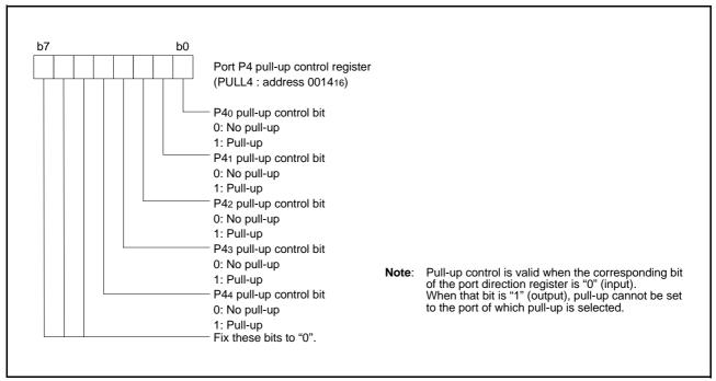
Fig 14. Structure of port registers (2)
