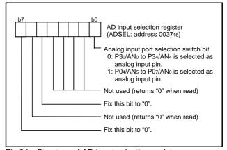
Fig 34. Structure of AD input selection register
