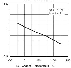
DRAIN TO SOURCE ON-STATERESISTANCE vs. CHANNEL TEMPERATURE
