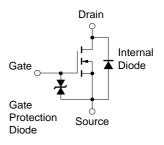
**Remark** The diode connected between the gate and source of the transistor serves as a protector against ESD. When this device is actually used, an additional protection circuit is externally required if a voltage exceeding the rated voltage may be applied to this device.
