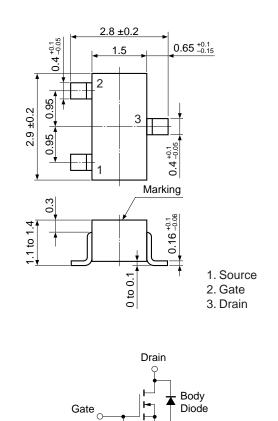
**Remark** The diode connected between the gate and source of the transistor serves as a protector against ESD. When this device actually used, an additional protection circuit is externally required if a voltage exceeding the rated voltage may be applied to this device.
