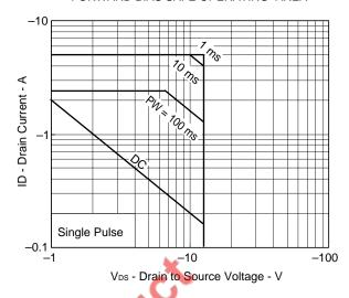
DRAIN CURRENT vs. DRAIN TO SOURCE VOLTAGE
