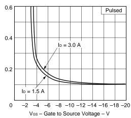
R<sub>DS(on)</sub> – Drain to Source On-State Resistance –  $\Omega$
