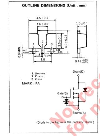
The 2SJ179, P-channel vertical type MOS FET, is a switching device which can be driven directly by the output of ICs having a 5 V power source.
