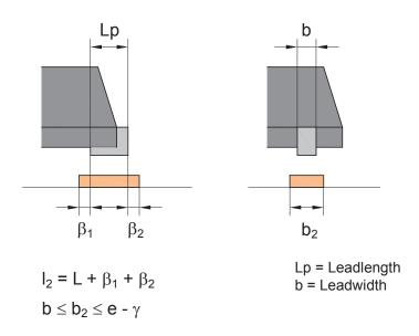
l<sub>2</sub> and b<sub>2</sub> can get by following formula and value e and b from package drawing figure and below parameter table.
