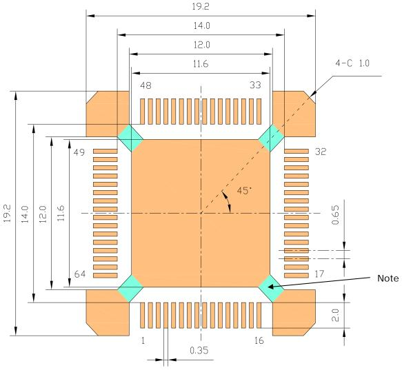
To ensure the amount of solder for pad area corresponding to the corner of heat spreader, we recommend set the area of solder resist or a silkscreen on PCB as preventing of solder outflow at reflow.
