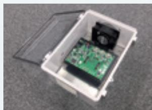
Allows testing using an inverter equivalent to circuits used in actual products.
