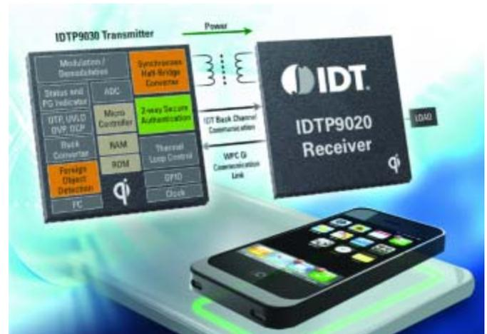
Figure 1: A wireless power charging system using IDT's IDTP9030 and IDTP9020 devices
