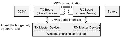
Figure 4.1 Evaluation system in MC1
