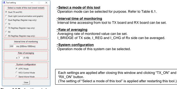
Figure 6.2 Tool setting window
