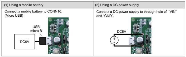
Connection method of power supply to WiQ-TX00-B00 Figure 1.2
