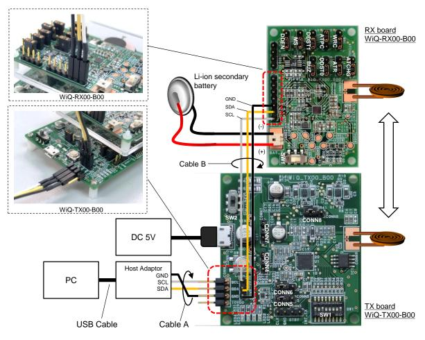
Figure 1.1 Connection of Wireless charging evaluation kit
