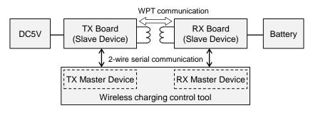
Figure2.1 Evaluation system in AT4
