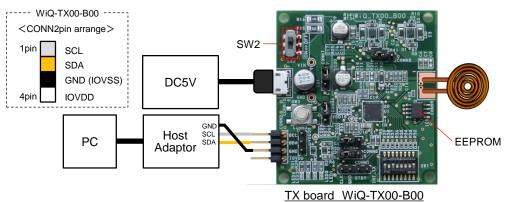
Figure 3.2 Connection in writing and reading EEPROM
