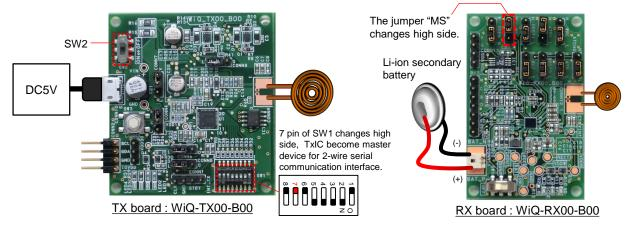
Figure 3.5 Connection of board in AT1
