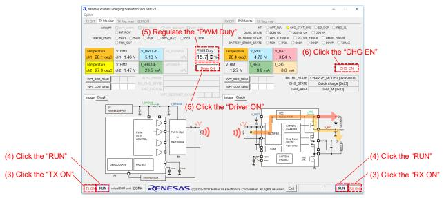
Figure 4.3 Control tool window in MCU Control Mode
