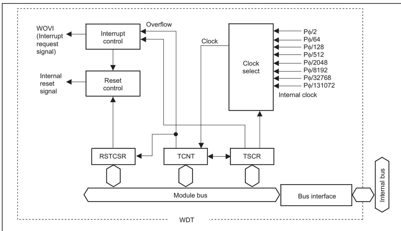
Figure 2 Block Diagram of Watchdog Timer
