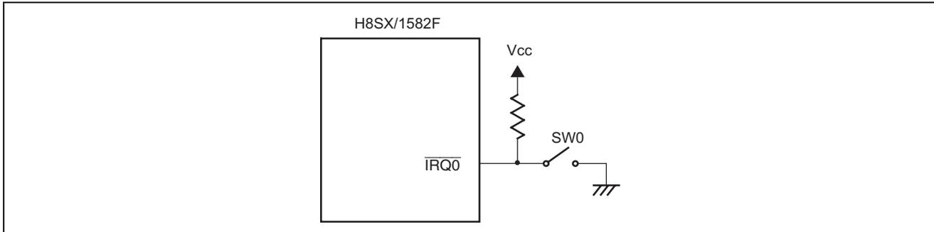
**Figure 1 Block Diagram of Connecting a Switch**
