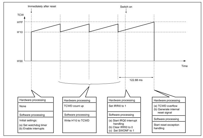
Figure 3.1 Operation Principle: Watchdog Timer Operation
