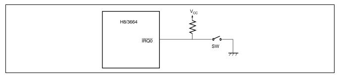
Figure 1.1 Example of Connecting Switch to IRQO Input Pin
