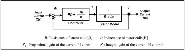
**Figure 3-2 Current Control System Model**
