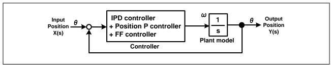
Figure 4-2 IPD controller model
