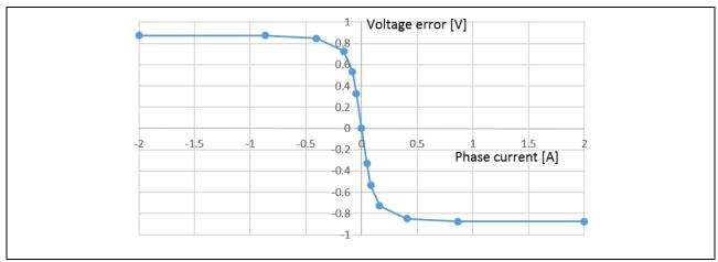
Figure 4-9 Current Dependence of Voltage Error (Example)
