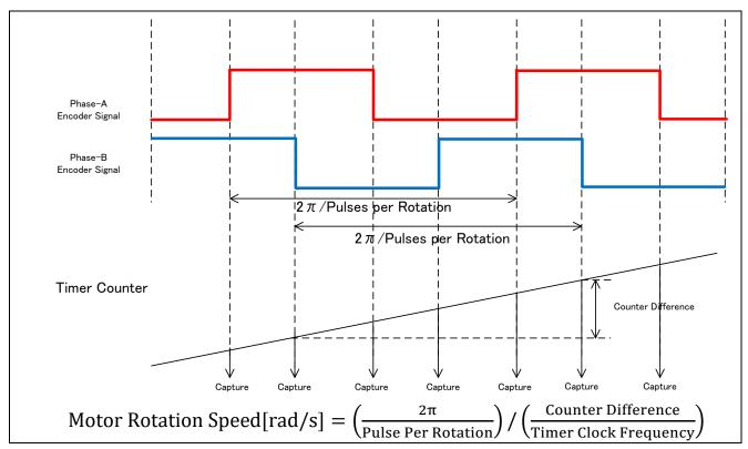
Figure 4-1 Speed Calculation Using Encoder
