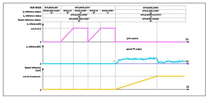
Figure 4-12 Startup Speed Control of Vector Control PMSM with Encoder Software
