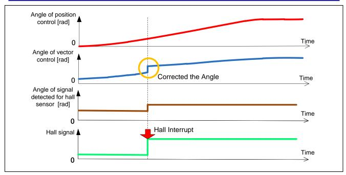
Figure 4-8 Magnet Position Detection Using Hall Sensor
