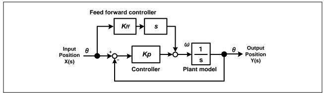
**Figure 3-4 Position Control System Model**
