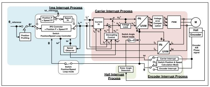
Figure 4-10 System Block of Vector Control with Encoder
