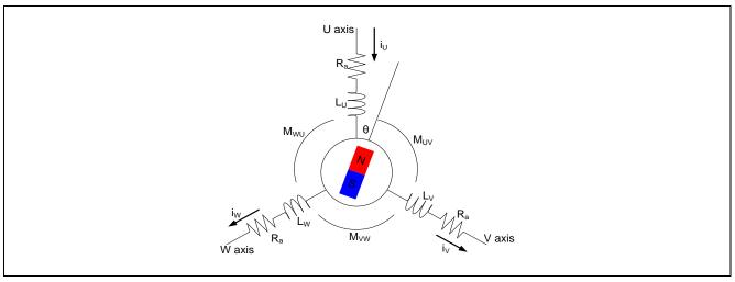
Figure 2-1 Conceptual Diagram of Three-phase Permanent Magnet Synchronous Motor
