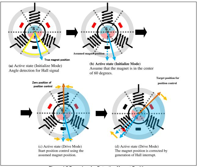
Figure 4-7 Procedure for Detecting Magnet Position
