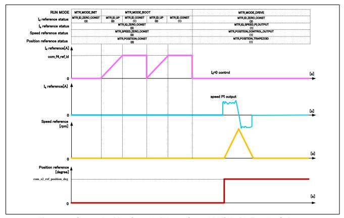
Figure 4-11 Startup Position Control of Vector Control PMSM with Encoder Software
