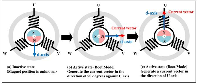
Figure 4-5 Determination of Position of Permanent Magnet
