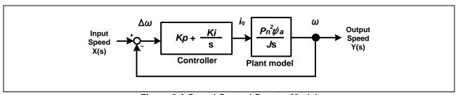
Figure 3-3 Speed Control System Model
