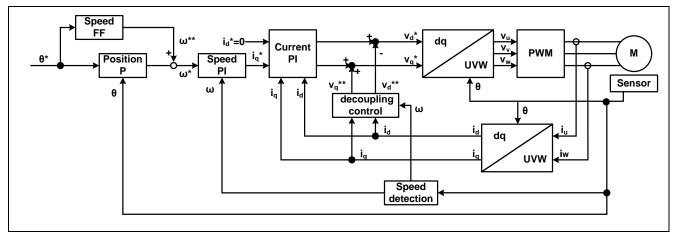
Figure 3-1 Vector Control System Block (Position Control)
