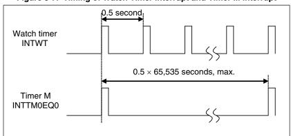
Figure 3-7. Timing of Watch Timer Interrupt and Timer M Interrupt
