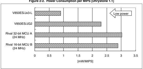
Figure 2-2. Power Consumption per MIPS [Dhrystone 1.1]
