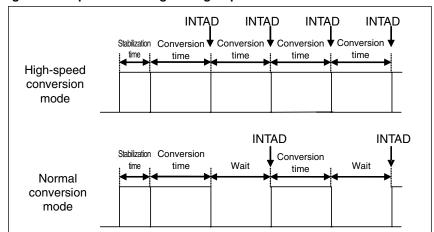
Figure 3-6. Operational Image of High-Speed and Normal Conversion Modes
