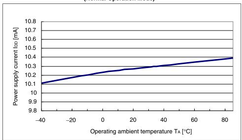
Figure 2-4. Relationship Between Operating Ambient Temperature and Power Supply Current (Normal Operation Mode)
