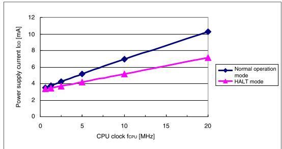
Figure 3-2. Relationship Between CPU Clock and Power Supply Current
