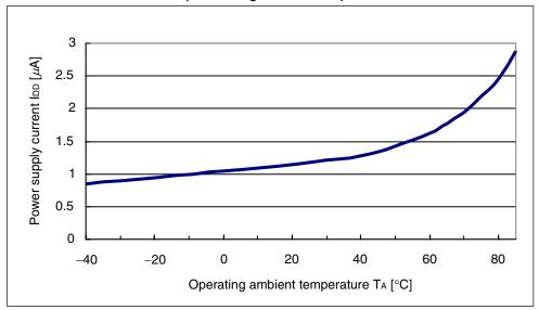
Figure 2-5. Relationship Between Operating Ambient Temperature and Power Supply Current (Low-Voltage STOP Mode)
