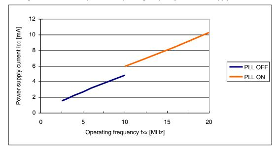
Figure 2-3. Relationship Between Operating Frequency and Power Supply Current
