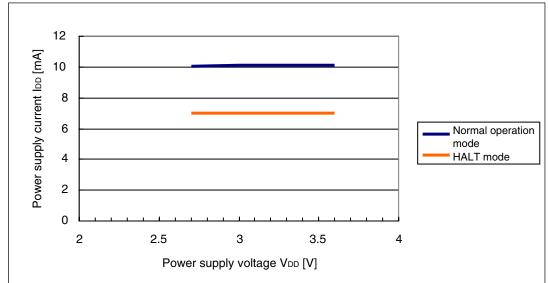
Figure 2-6. Relationship Between Power Supply Voltage and Power Supply Current at 20 MHz Operation
