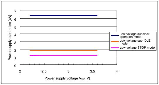
Figure 2-7. Relationship Between Power Supply Voltage and Power Supply Current in Low-Voltage Mode
