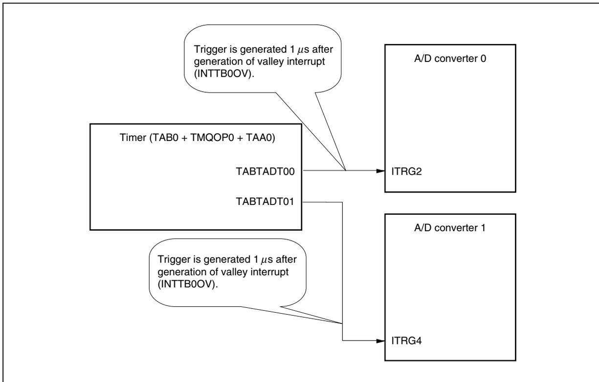
With the 3-phase PWM driver, the timing of conversion start trigger of A/D converters 0 and 1 is the same. To change the conversion start time, set the TAA0CCR0 and TAA0CCR1 registers in accordance with the above expression.
