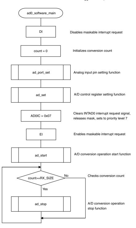
Software trigger mode (continuous select mode, 1 buffer) (2/2)
