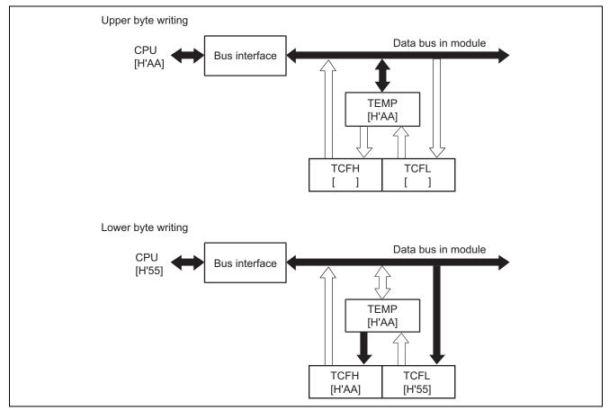
Figure 3 TCF Write Operation
