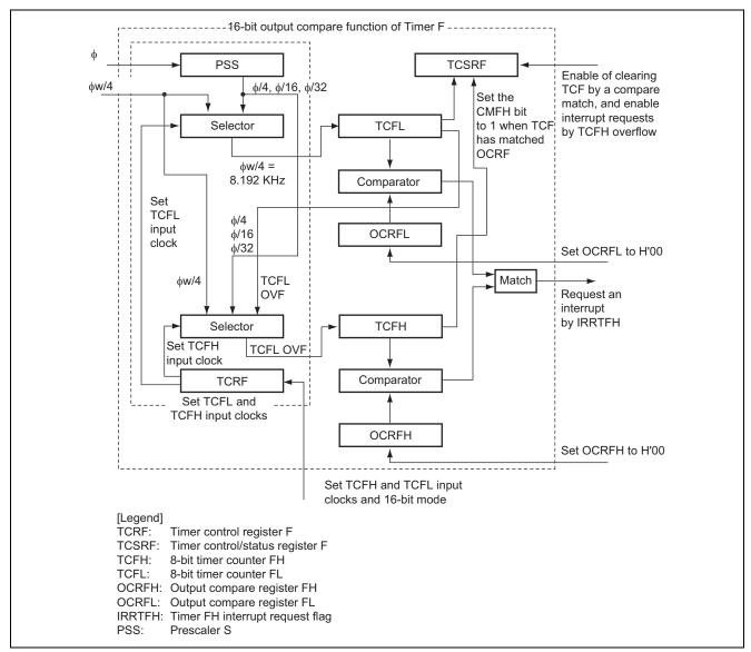
Figure 2 Block Diagram of 16-Bit Output Compare Function of Timer F
