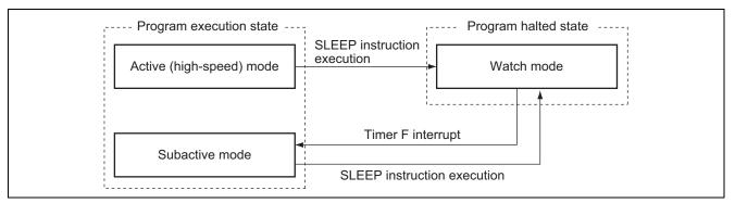
Figure 1 Diagram of Mode Transitions for this Sample Task
