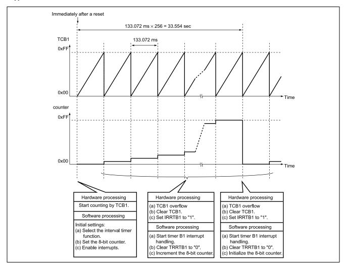
Figure 3.1 Operation Principle
