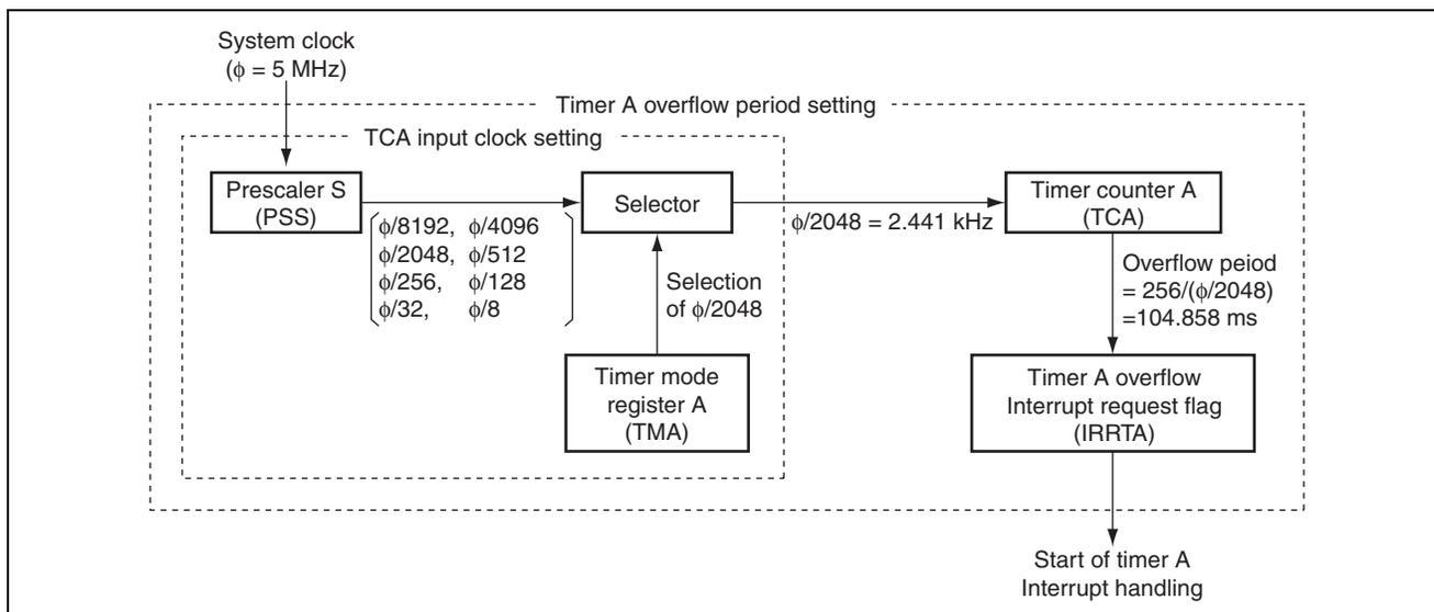
**Figure 2.1 Block Diagram of Timer A Interval Function**
