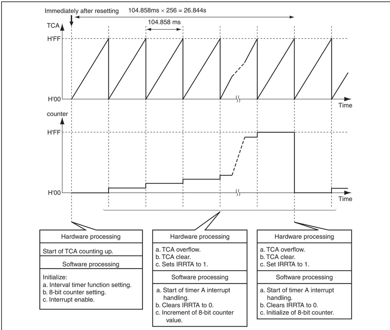
Figure 3.1 Operation Principle of Counting up the 8-bit Counter by the Timer A Interval Function
