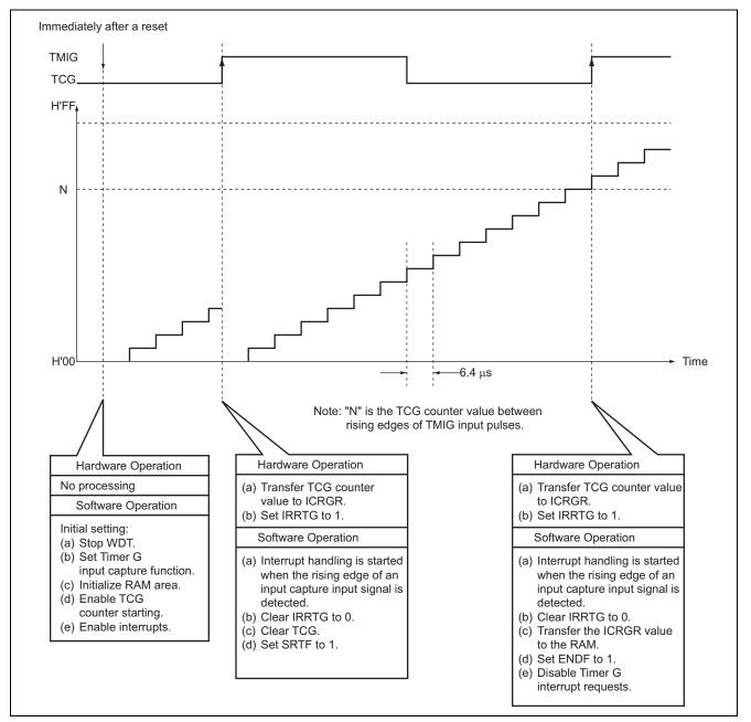
Figure 3 Principle of Operation of Pulse Period Measurement by Timer G Input Capture Function
