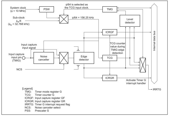
Figure 2 Block Diagram of Timer G Input Capture Function
