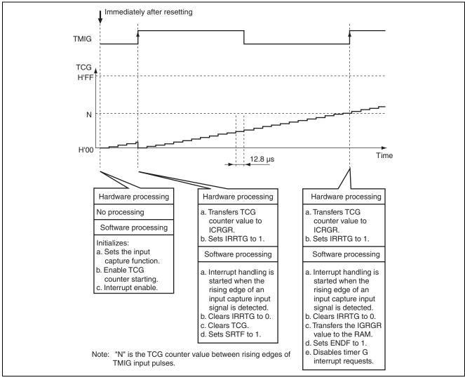
Figure 3.1 Operation Principle of Pulse Period Measurement by Timer G Input Capture Function
