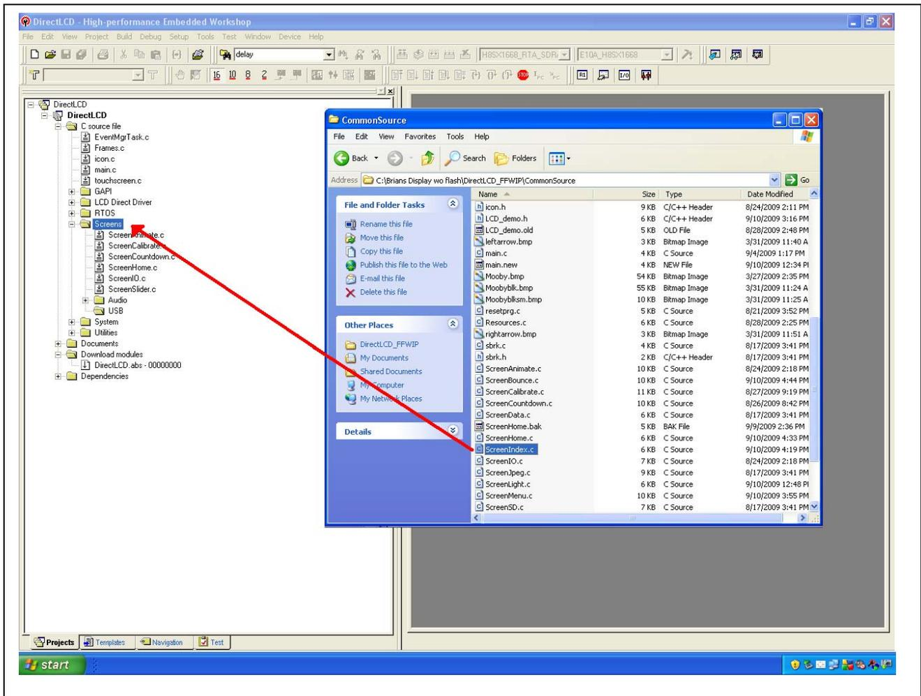
**Figure 3: Adding “ScreenLight.c” to the Direct LCD demo project in HEW**
