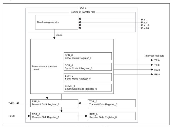
Figure 3 Block Diagram of SCI\_0
