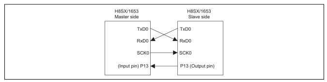
Figure 1 Clock Synchronous Serial Transmission and Reception
