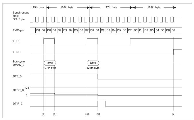
Figure 7 Timing of Transmission End
