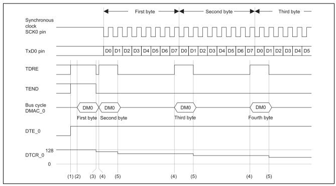
Figure 6 Timing of Transmission Start
