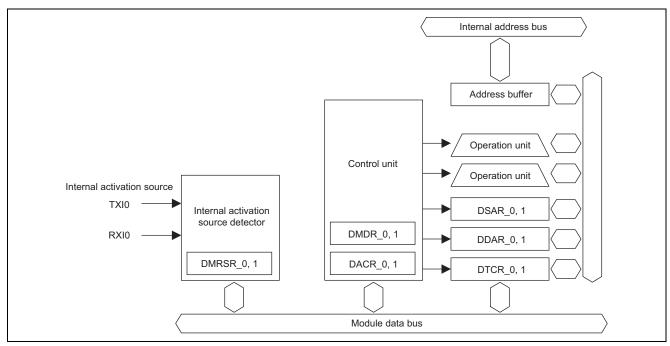
Figure 4 Block Diagram of the DMAC
