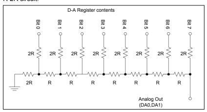
Figure 1 Example DAC R-2R Circuit
