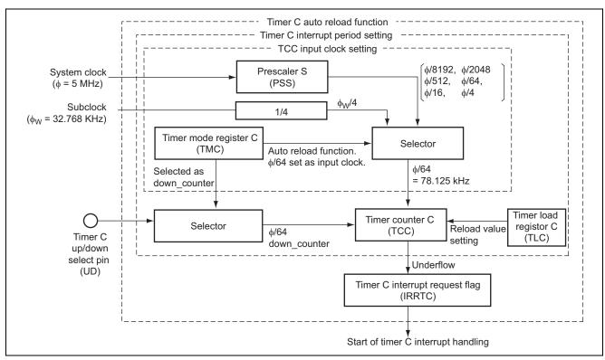
Figure 1 Block Diagram of Timer C Auto-Reload Function
