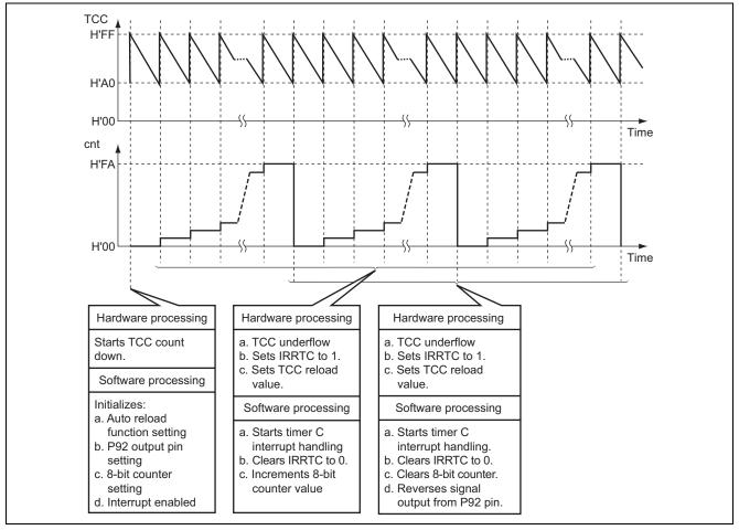
Figure 2 Operation Principle of Interrupt Period Setting by Timer C Auto-Reload Function
