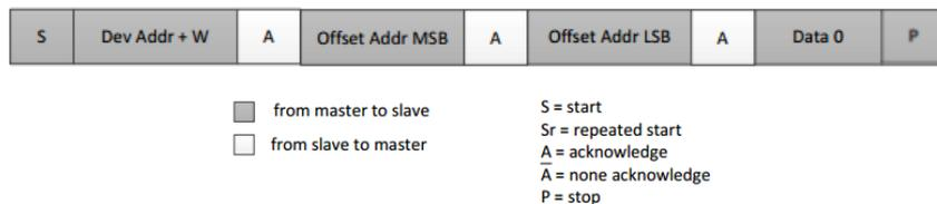
Figure 1. Single-Byte Write
