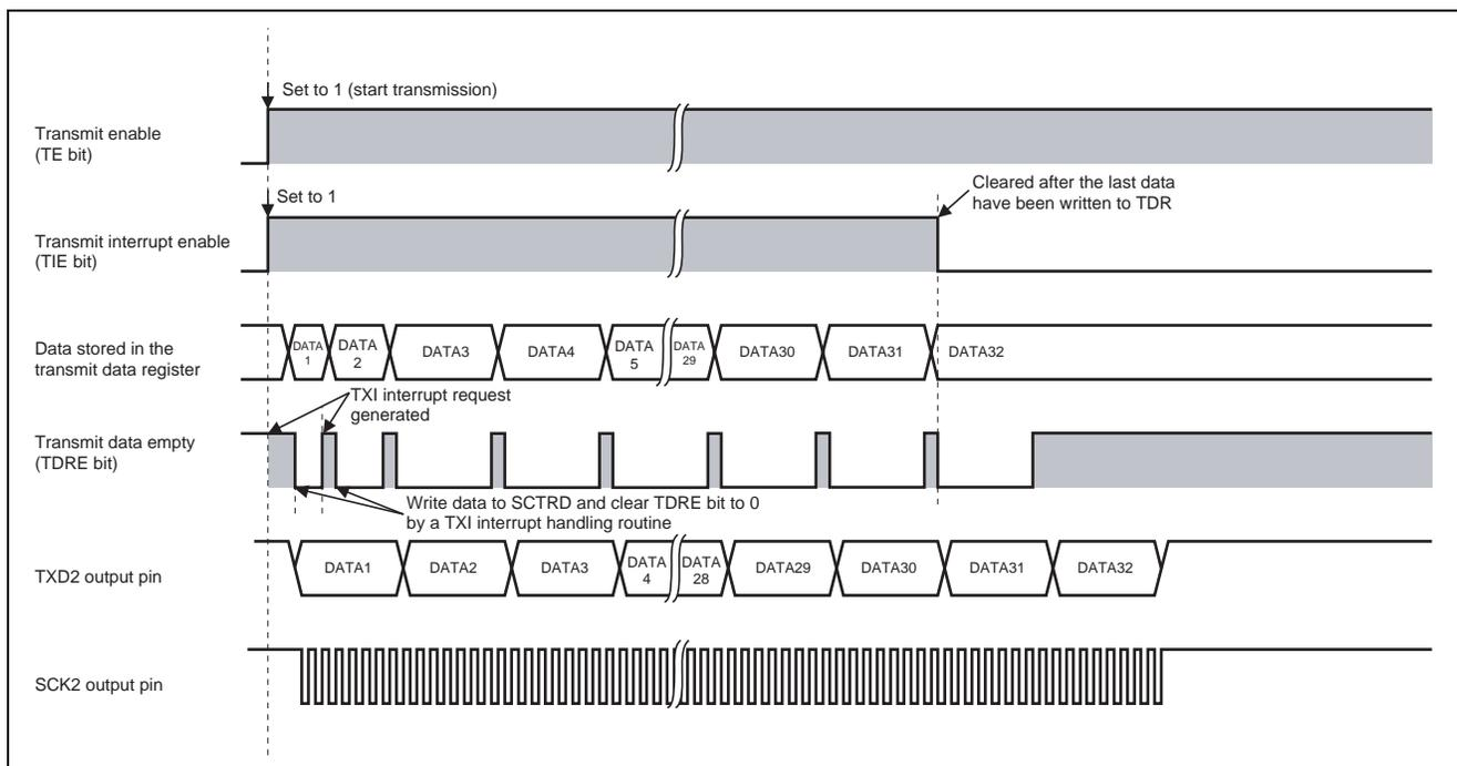
**Figure 3 Operations for Data Transmission**
