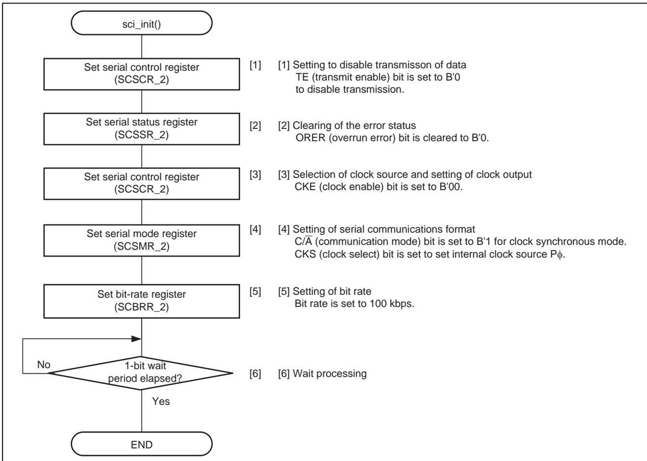
**Figure 6 Flow for Initialization of Data Transmission in Clock Synchronous Mode**
