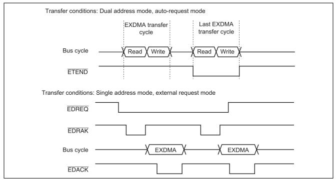
Figure 4 Example of Timing in Normal Transfer Mode
