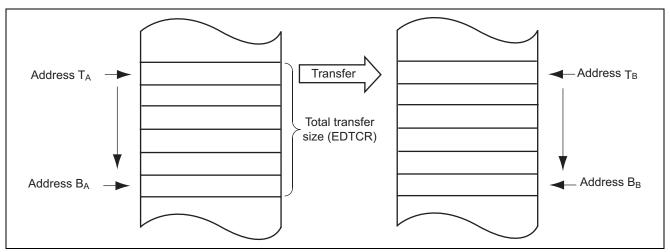
Figure 5 Example of Operation in Normal Transfer Mode
