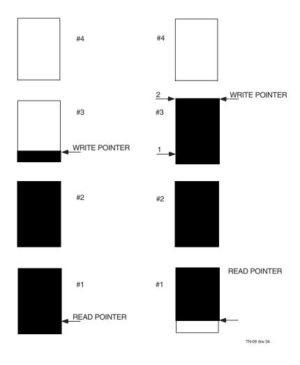
Case 1: In the cascaded FIFO arrangement, the write pointer has just written to FIFO #3 and the flag defined by the f1 equation would be asserted at the half-full point.
