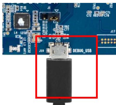
2. Connect the other end of the USB cable to the USB port on your PC. LED4 on the SK-S7G2 lights green indicating the SK-S7 is now properly connected to the PC.
