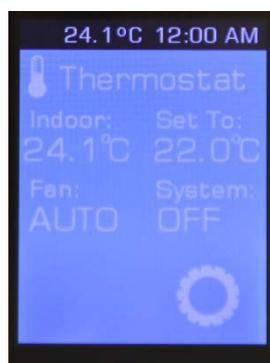
3. Tap the settings icon (looks like a gear) on the bottom right to make adjustments to the system including Units, Time and Date.
